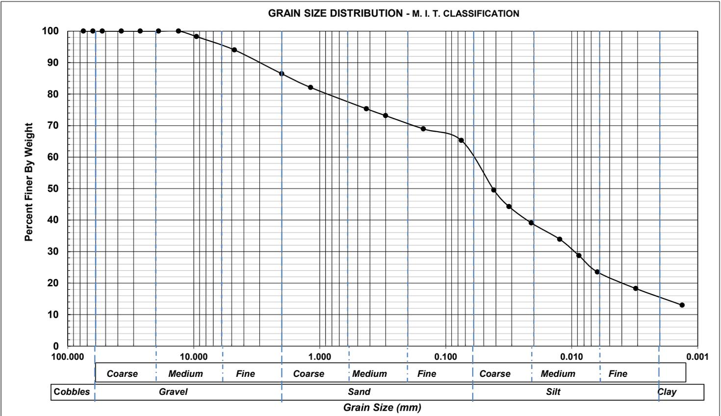
GRAIN SIZE ANALYSIS - HYDROMETER TEST
