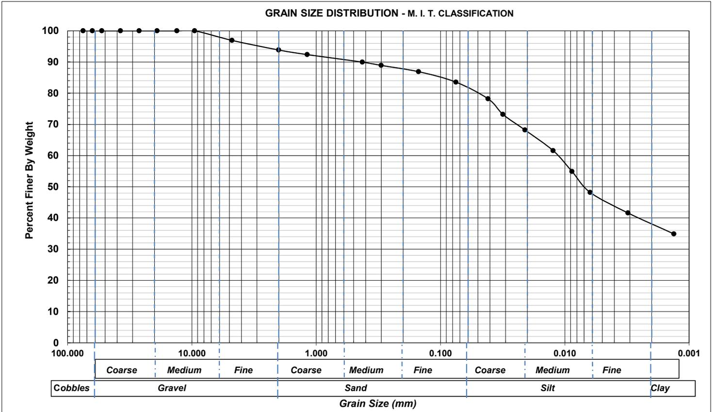
GRAIN SIZE ANALYSIS - HYDROMETER TEST
