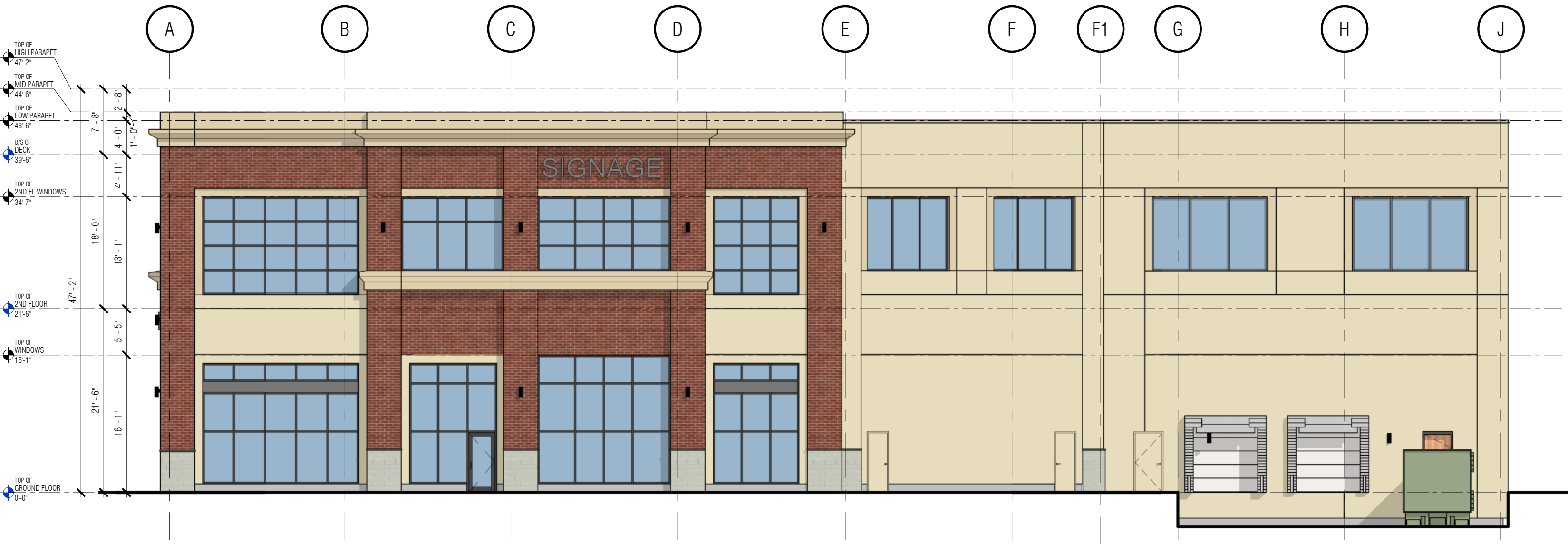
1 BLDG F - WEST ELEVATION 3/32" = 1'-0"
