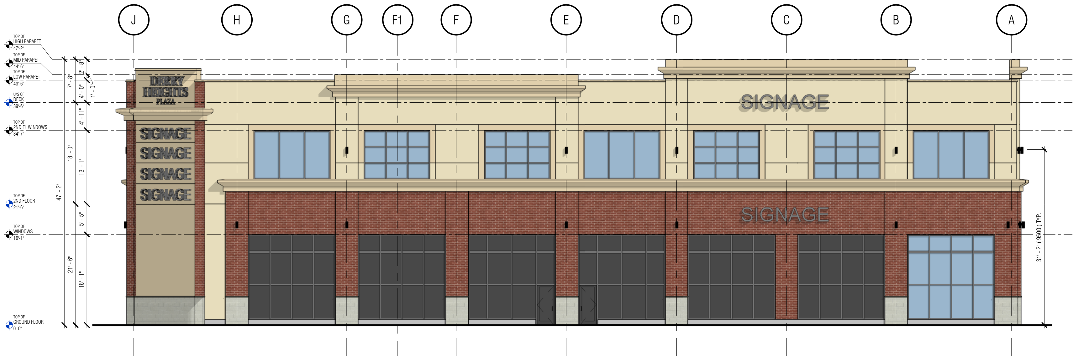
7 BLDG F - EAST ELEVATION AF3.0 3/32" = 1'-0"
