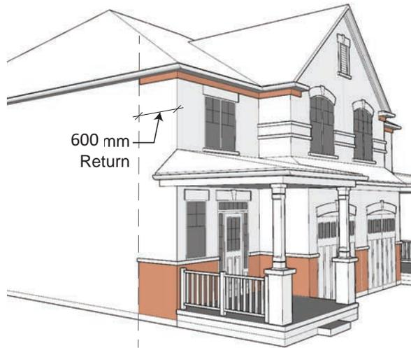
Front façade detailing (i.e. stone, stucco, frieze/cornice) shall return a minimum of 600mm along the side wall
