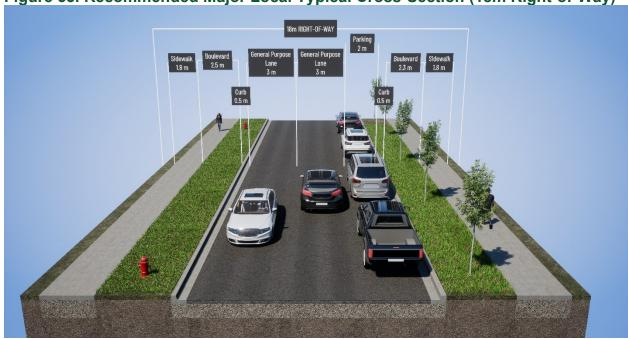
Figure 53. Recommended Major Local Typical Cross-Section (18m Right-of-Way)
