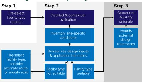
Figure 38. Three-Step Facility Selection Tool
