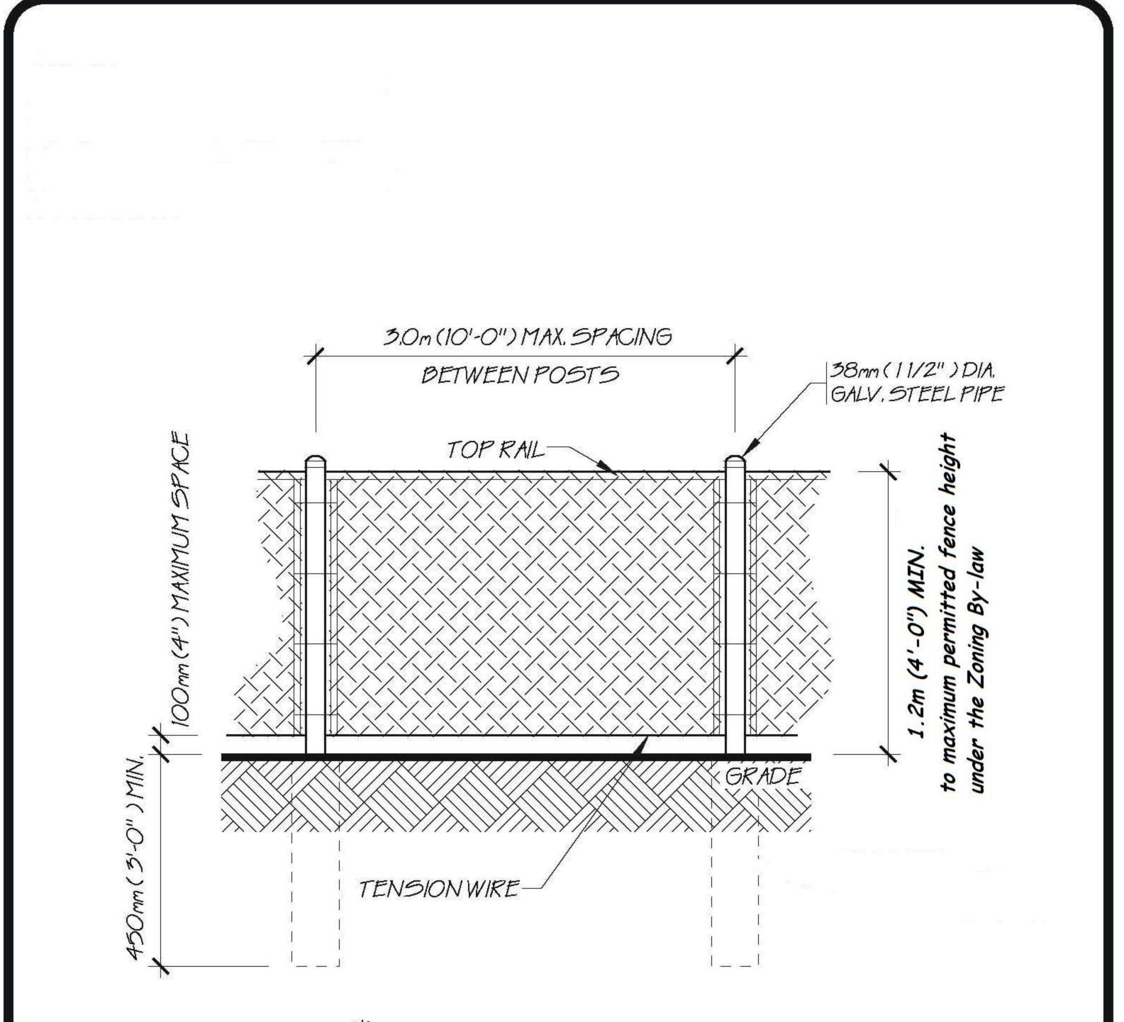
\*CHAIN LINK FENCING WITH LINKS LARGER THAN 38mm (11/2") SHALL EXTEND A MINIMUM OF 1.8m (6'-0") ABOVE GRADE
